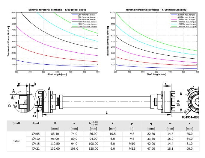
The installed length L is dependent on the application and is limited by the type of design and maximum speed.
