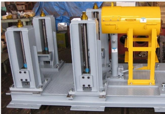
Engine Mounts and Mobile Universal Base
