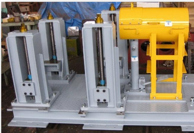
Engine Mounts and Mobile Universal Base
