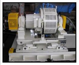
Especially in case of harsh condition, continuous durability test, or etc., since bearing and sealings are damaged quickly, periodic replacement of these are required. After the maintenance, we in detail confirm the condition of products such as calibration inspection, running inspection, and etc before delivery. The testing devices which pass the rigid company criteria can be delivered to customers again.
