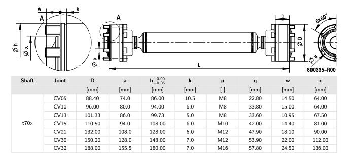
The length L is dependent on the application and is limited by the type of design and maximum speed. Higher speeds are available on request.
